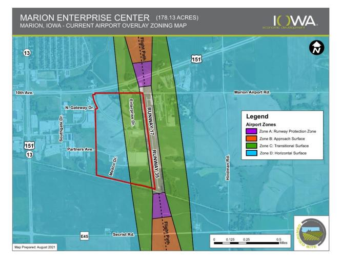
Zone C (Transitional Surface) - The transitional surface extends outward and upward at right angles to the runway centerline and extends at a slope of seven feet horizontally for each one foot vertically (7:1) from the sides of the primary and approach surfaces. The transitional surfaces extend to the point at which they intercept the horizontal surface at a height of 150 feet above the established airport elevation.
