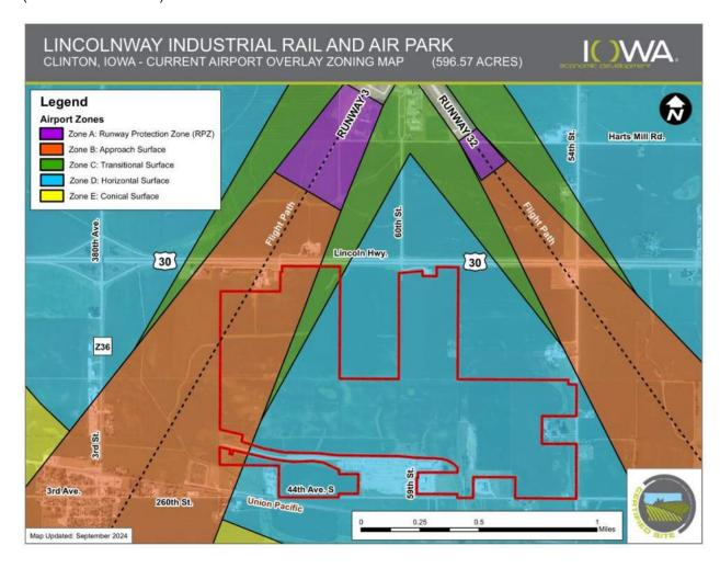
**Zone B: Approach Surface** is a critical overlay surface that reflects the approach and departure areas for each runway at an airport. The size of Zone B is predicated upon the type of approach (visual, non-precision, or precision) that a specific runway has and the type/size of aircraft utilizing the runway.
