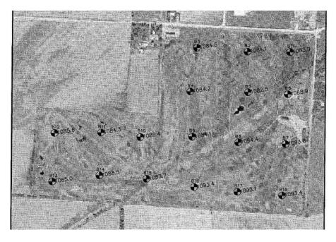
An additional Geotechnical Engineering Report was completed on the Jorgensen and Moore properties and included nine test broindgs to depths of 26 to 36.5 feet below existing grades. Certified Testing Services (CTS) recommends using Seismic Site Class D for the site.
