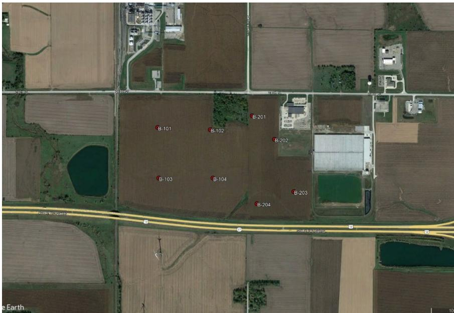
An additional Report of Preliminary Geotechnical Exploration was completed on the eastern portion of the Newman Farms property and included 4 borings to depths of 15 to 26 feet below existing grades. American Engineering Testing recommends using Seismic Site Class D for the site. *Note: For both reports, the consultant relied on their knowledge of regional geology and the results of the borings to determine Seismic site class.*
